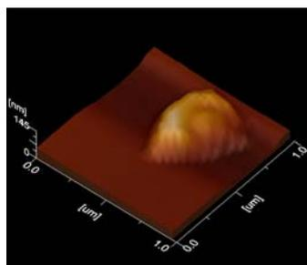
**Figure 4.** 10 Å Cu deposition on Si(111) at 750°C
