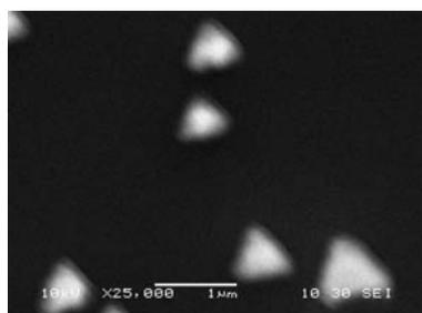
**Figure 1.**  $60\text{\AA}$  Cu deposition on Si(111) at  $750^\circ\text{C}$
