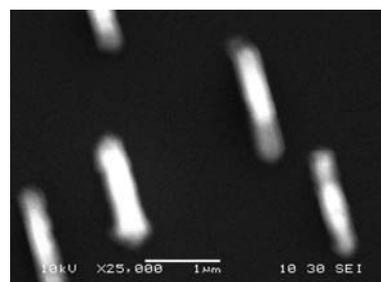
**Figure 3.**  $60\text{\AA}$  Cu deposition on Si(110) at  $750^\circ\text{C}$
