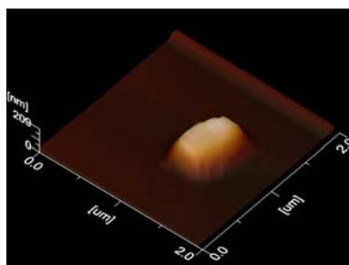
**Figure 5.** 10 Å Cu deposition on Si(100) at 750°C
