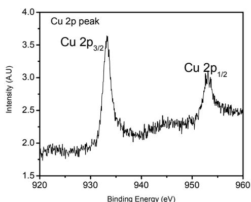
**Figure 7.** XPS spectra of Cu nanostructure deposited on Si(111) substrate for Cu 2p peak
