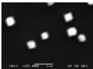
**Figure 2.**  $60\text{\AA}$  Cu deposition on Si(100) at  $750^\circ\text{C}$
