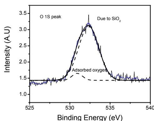
**Figure 8.** XPS spectra of Cu nanostructure deposited on Si(111) substrate for oxygen 1s peak
