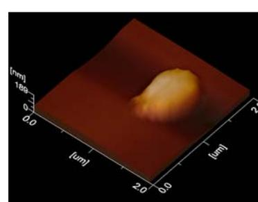
**Figure 6.** 10 Å Cu deposition on Si(110) at 750°C
